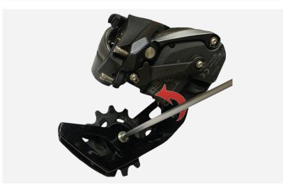
**4.** Replace the SRAM pulley with the remaining Nova pulley. Screw it with the M5x16 screw provided in the box and the 5mm Allen key.
