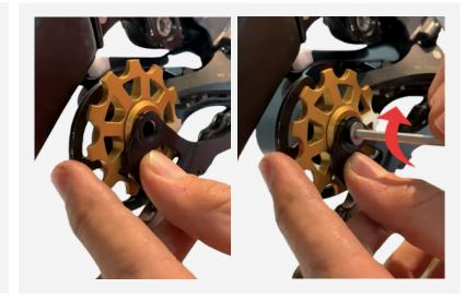
**3.** Remove the second Shimano pulley by using the 5mm Allen key.
