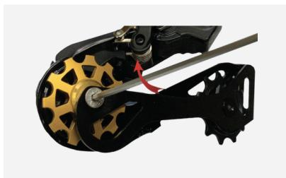
**3.** Unscrew the second pulley by using the 5mm Allen key.
