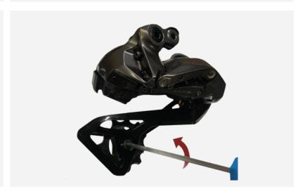
**4.** Insert the Nova Ride pulley and screw it with the second M5x16 screw provided in the box.
