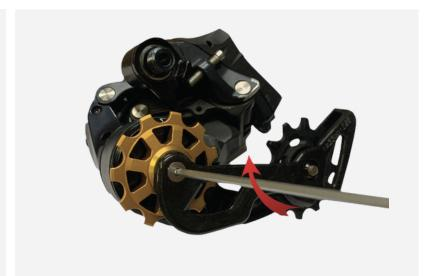
**3.** Remove the second SRAM pulley by using the 5mm allen key.
